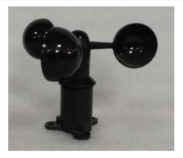
Wind Speed Sensor is designed with rugged components stand up to hurricane - force winds, yet are sensitive to a light breeze. Includes sealed bearings for long life. The range and accuracy specifications have been verified in wind - tunnel tests. In areas where icing of the anemometer is a problem, drip rings deflect water from the joint between moving parts.
