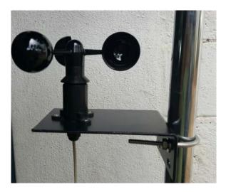
Mount the sensor On a Pipe with 1.5" Dia using the U bolt provided
